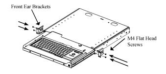
Step 2 Mounting DR4 into front of 2/4 Post Relay Rack.
