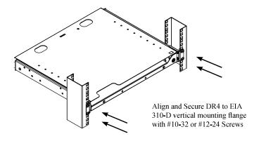
Step 3 Installing 5" Center Bracket
