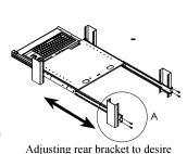
Adjusting rear bracket to desire depth in the cabinet.
