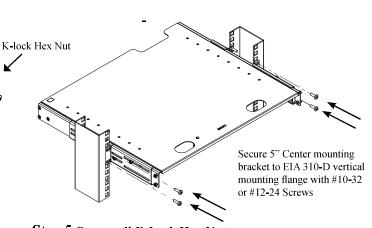
Step 2 Mounting DR4 into front of 2/4 Post Relay Rack.
