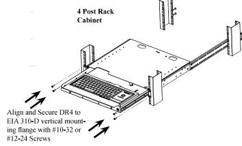
Step 4 Installing Left side rear-mount bracket
