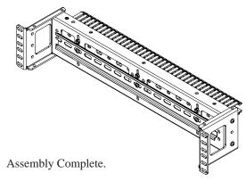
Step 2 Install PVC Wire Duct using hex nuts
